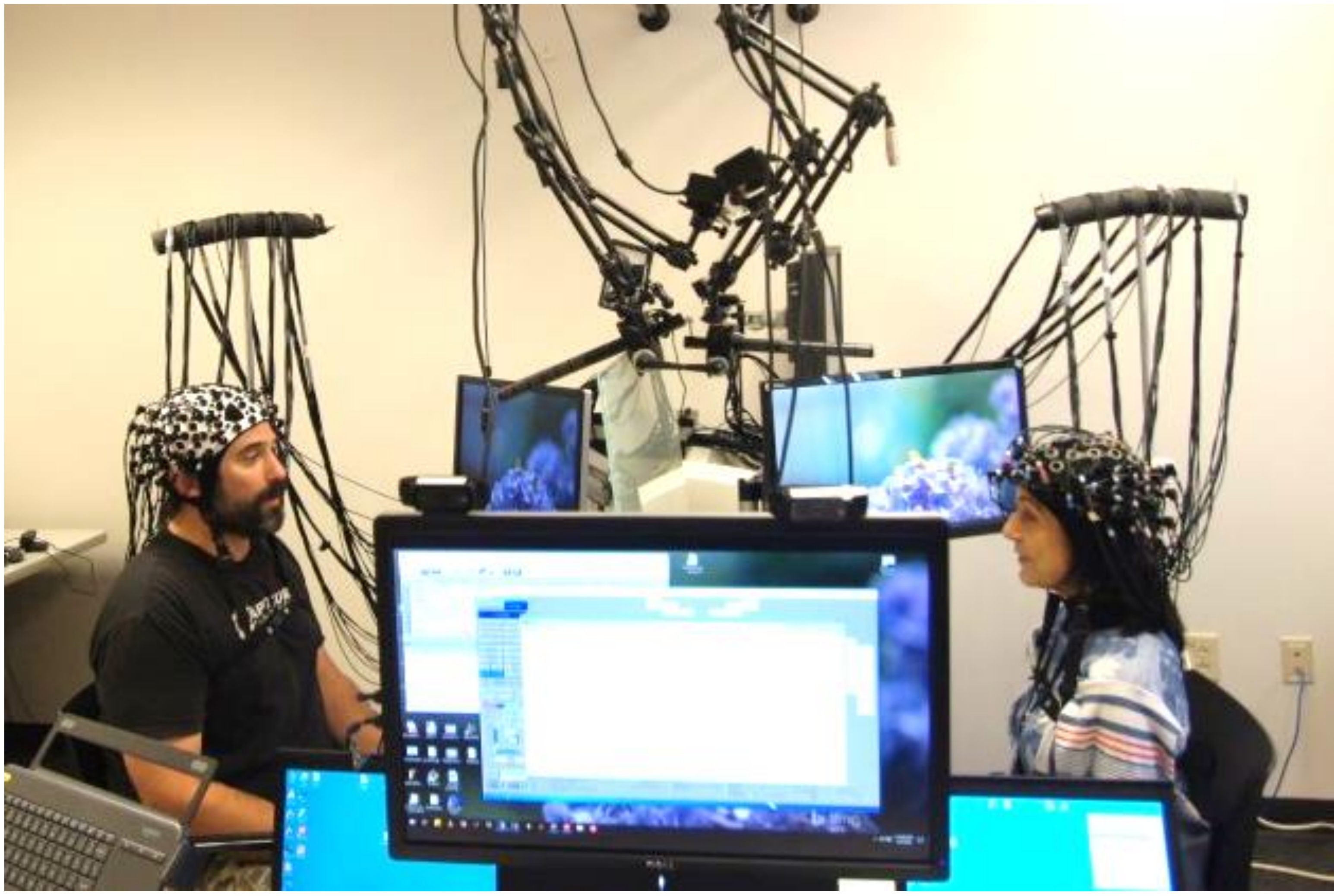
Figure 1. Hyperscanning set up for recording live speech while acquiring functional near infrared spectroscopy (fNIRS) signals during debate under contrasting agreement and disagreement conditions. Talking and listening epochs alternated every 15 sec. Debate topics were assigned based on previously surveyed agree/disagree opinions of the partners.
